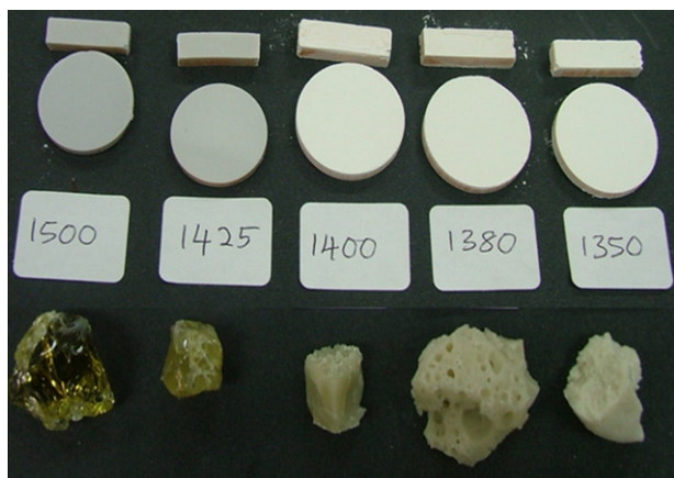
Fig. 13. Appearance of glass and glass–ceramic of samples melted at different temperature.
