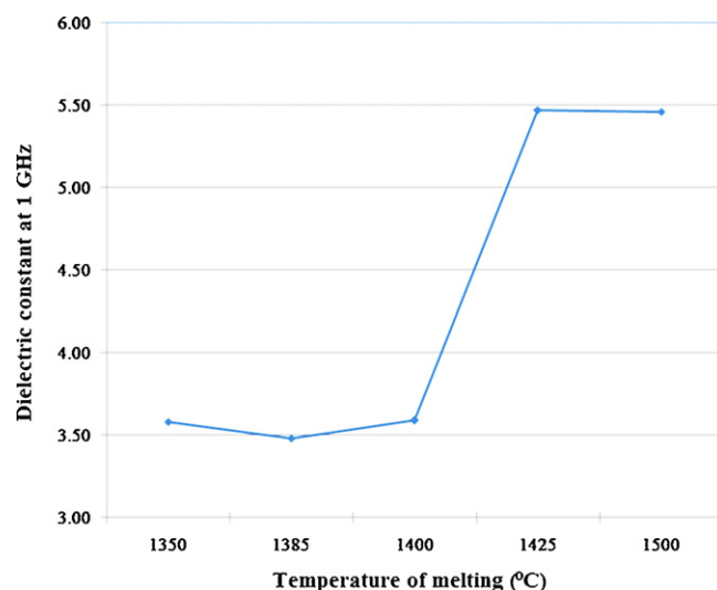
Fig. 7. Effect of melting temperature on dielectric constant measured at frequency 1 GHz.
